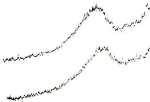
Fig.4 Perlite X-ray diffraction patterns. a) Upper –raw perlite; b) lower – perlite sintered at 900 o C
